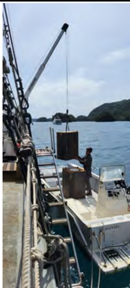
In preparation for sailing over the coming year, we're installing new holding tanks for the gray and black water from the ship's forward head.
