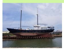
Three years from her last dry docking, we found it necessary to return to the Philippines with the ship for another haul-out. The problem we faced was a leaking stern tube which was admitting far too much water into the bilge causing us to have to pump out two to three times, daily. The photo at the left shows her up on the rails of Colorado Shipyard, Cebu City, Pl. We were 11 days hauled out and two weeks in transit.
