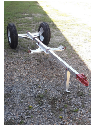
This modular, two-wheel trailer is a special design by our USA based co-laborer in missions, Jerry Hardman, Fordyce, AR. It is making it's way to Micronesia now for use behind our Honda ATV, hauling loads of supplies.
